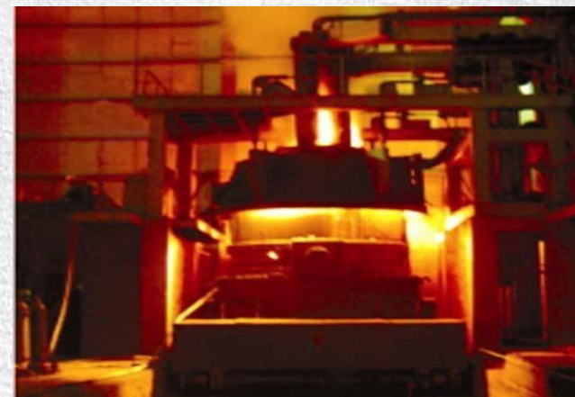
Two Ladle Refining Furnace
