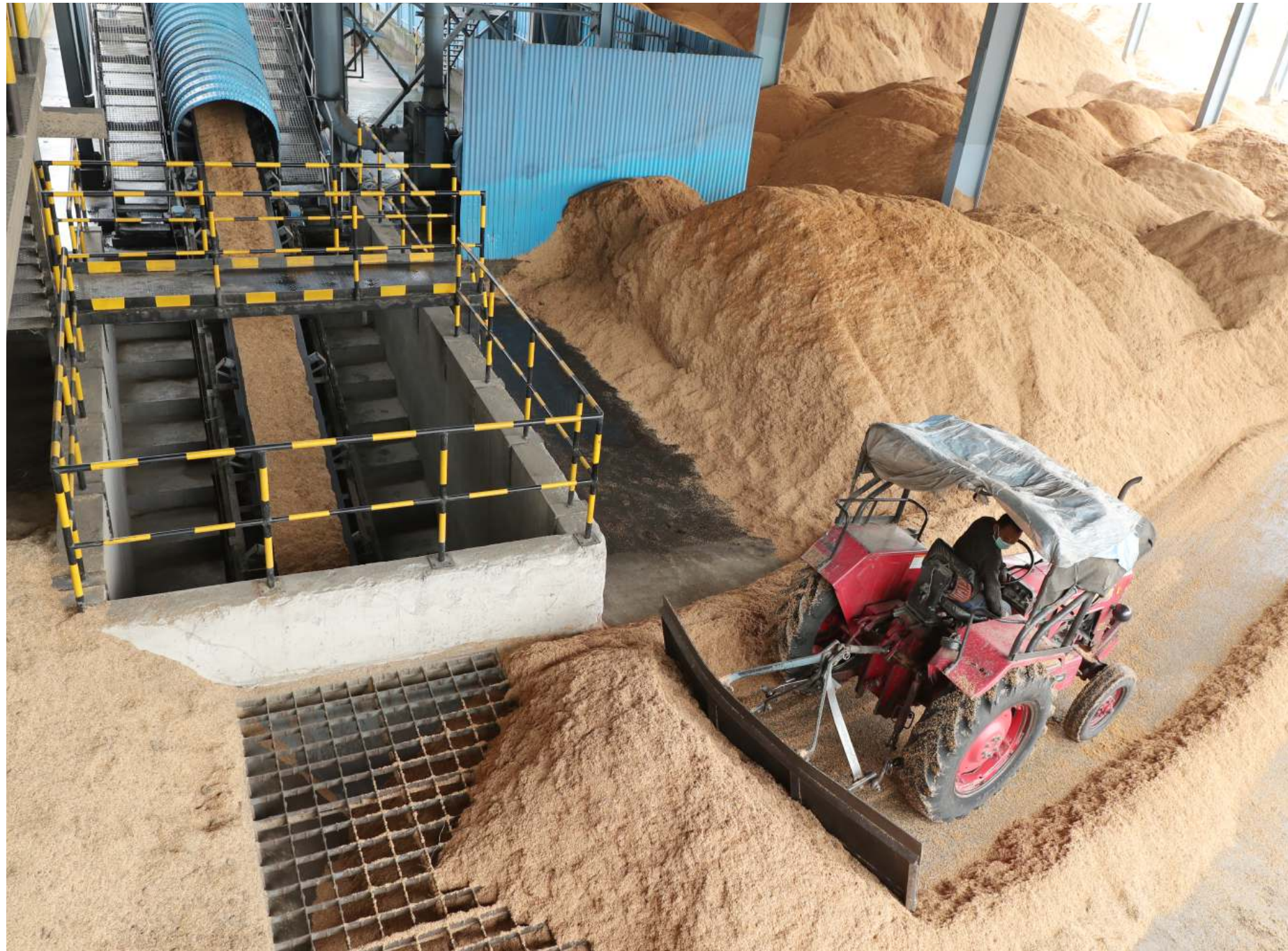
Utilisation of husk as fuel in power plant boiler to reduce coal usage
