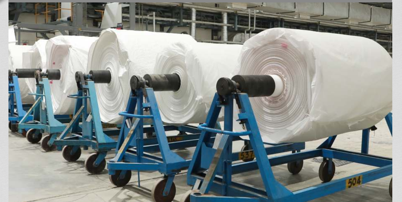
1 Single use plastic sheets replaced with reusable HDPE sheets for covering
